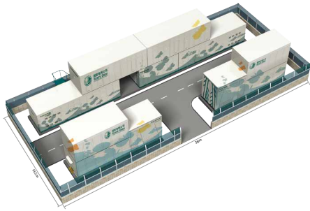
3D view of HV GIS module
