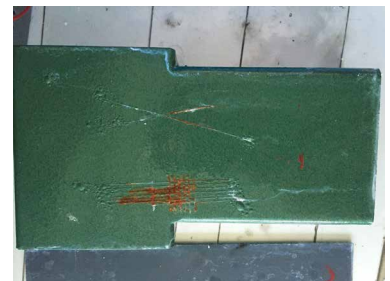
Final paint layer 750 hrs salt fog test
