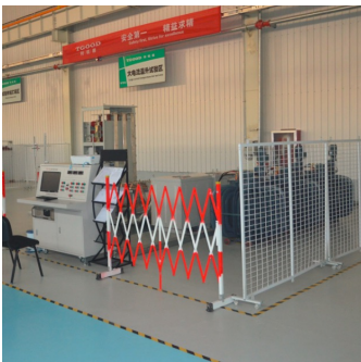
Temperature rise test facility up to 7000 A
